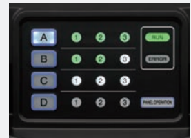
Signaled by white light for properly set cassettes, blinked white light for not properly set cassettes, green light for the completion of scanning.
